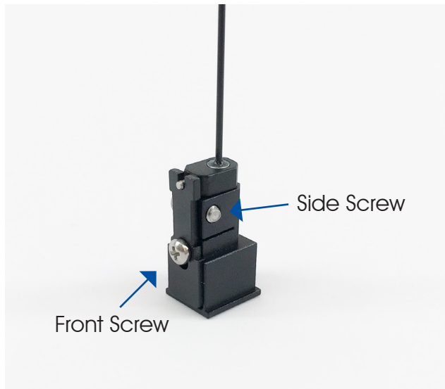
Figure 3. OASIS implant headmount with fiber inserted. Side screw locks the fiber in place. Front screw locks fiber focus.
