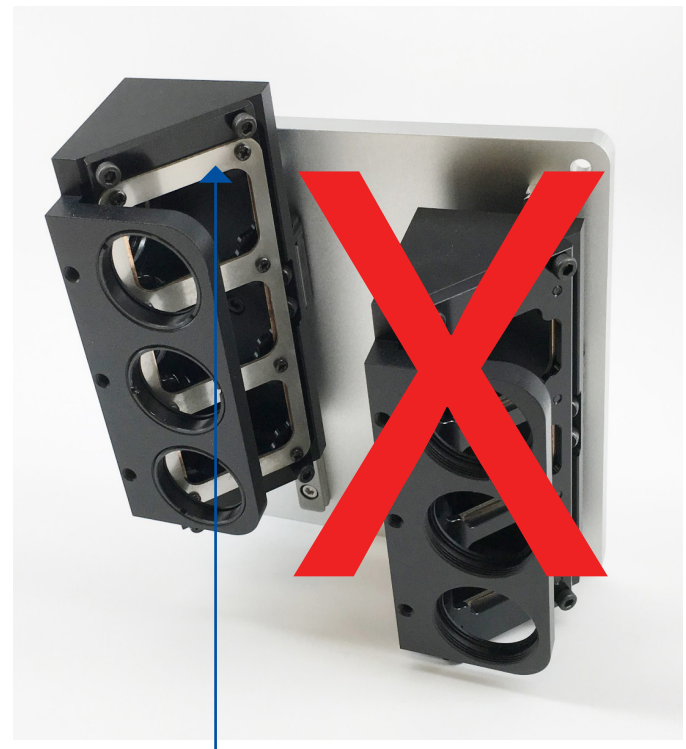
Incorrect. Dichroic cover facing outside.
