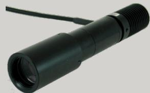
PLS high-uniformity, precision close-range LEDs have a minimum working distance of 75mm, being able to produce a 10mm diameter spot at such distance. These LEDs also have a maximum working distance of 100mm, producing a spot 17mm in diameter.
