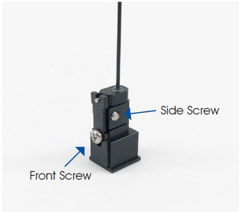
Figure 3. OASIS implant headmount with fiber inserted. Side screw locks the fiber in place. Front screw locks fiber focus.
